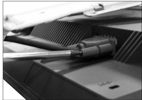
1. Remove the screw for the signal cable. 2. Pull out the signal cable.
